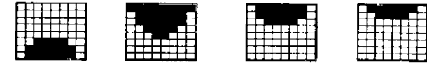
Figure 3. Parameterization of defects during simulation : a) OD 6mm; b) ID 9mm; c) ID 6mm; d) ID 3 mm
